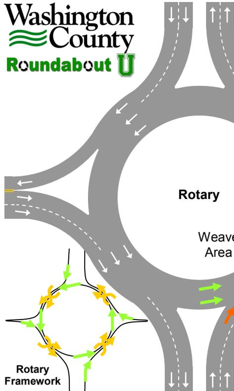
These drawings show how traffic streams interact at a *rotary* versus a roundabout.
